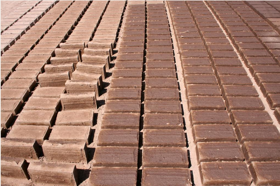
Adobe bricks in the process of drying, made in the open air.
